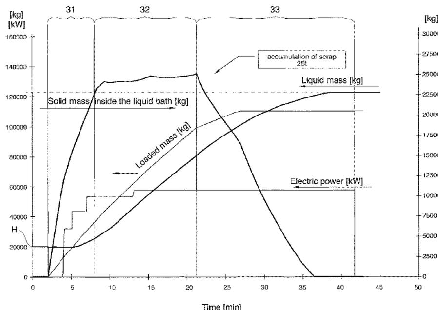
load said metal material into said shell, said method comprising at least a step of loading said metal material into said shell by means of said feed means, a melting step in which said metal material is melted, and a subsequent tapping step in which the molten metal material is tapped.
