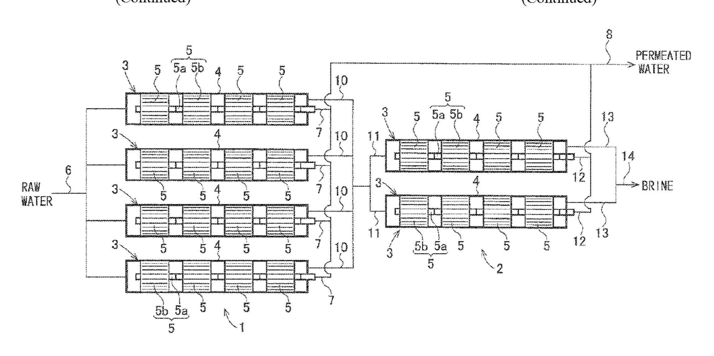
an end of a final stage of the high-pressure reverse-osmosis-membrane separation device is 2.1 m<sup>3</sup>/(m<sup>2</sup>·D) or more.
