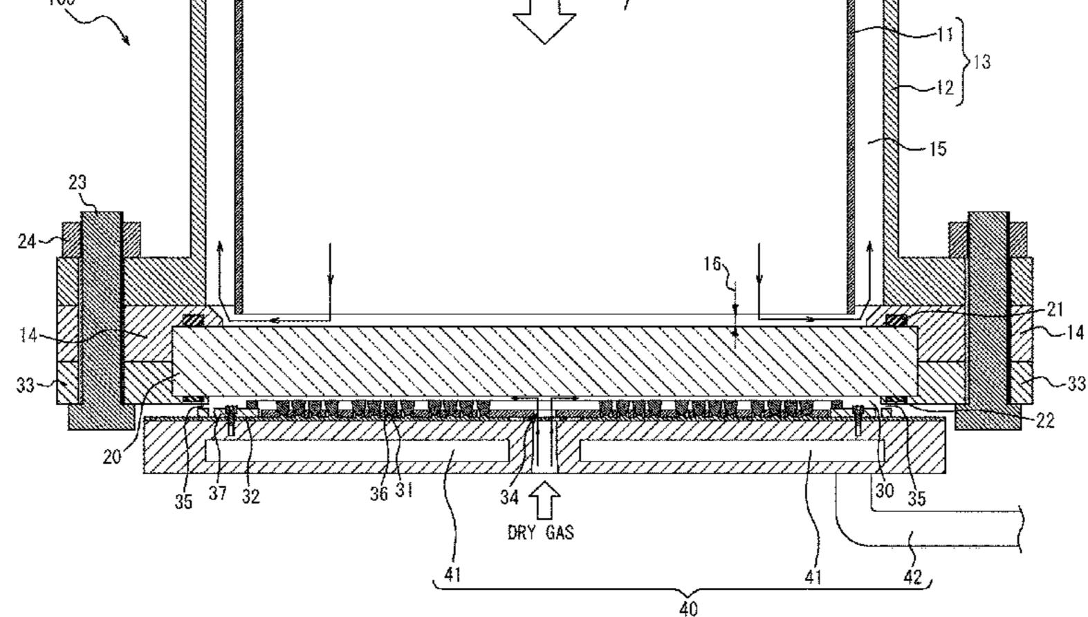
dry gas, and light emitting surfaces of the plurality of LED elements 31 are exposed to a space in the LED element housing chamber 30.
