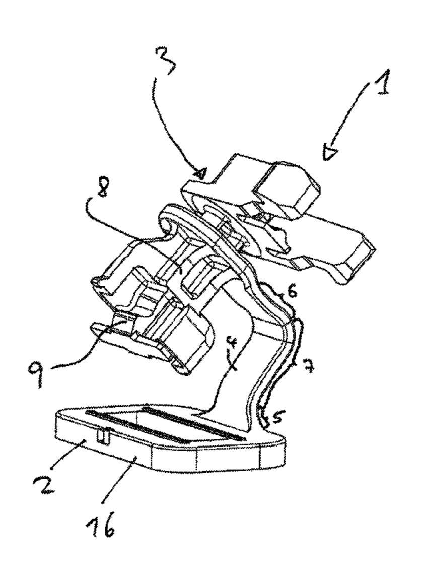
wherein a spacer is situated between the first connector and second connector, and a projection of the spacer protrudes into the space inside the bent portion of the restraining band in the normal operating state of the fastener.
