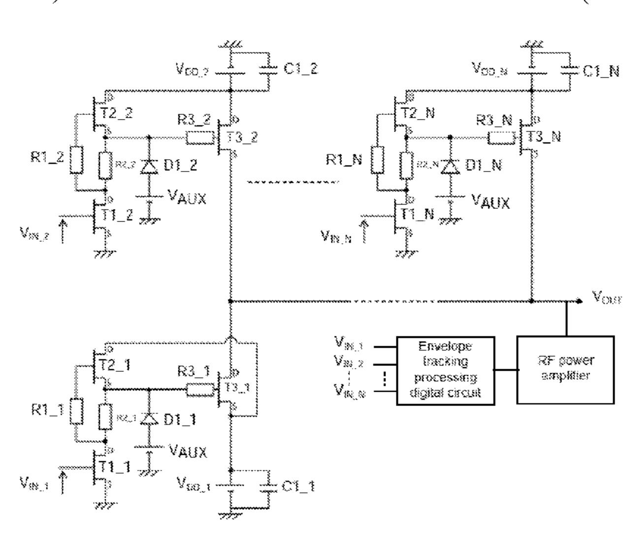
(VDD\_2) distributed between the lower (VDD\_1) and upper (VDD\_N) supply voltages.
