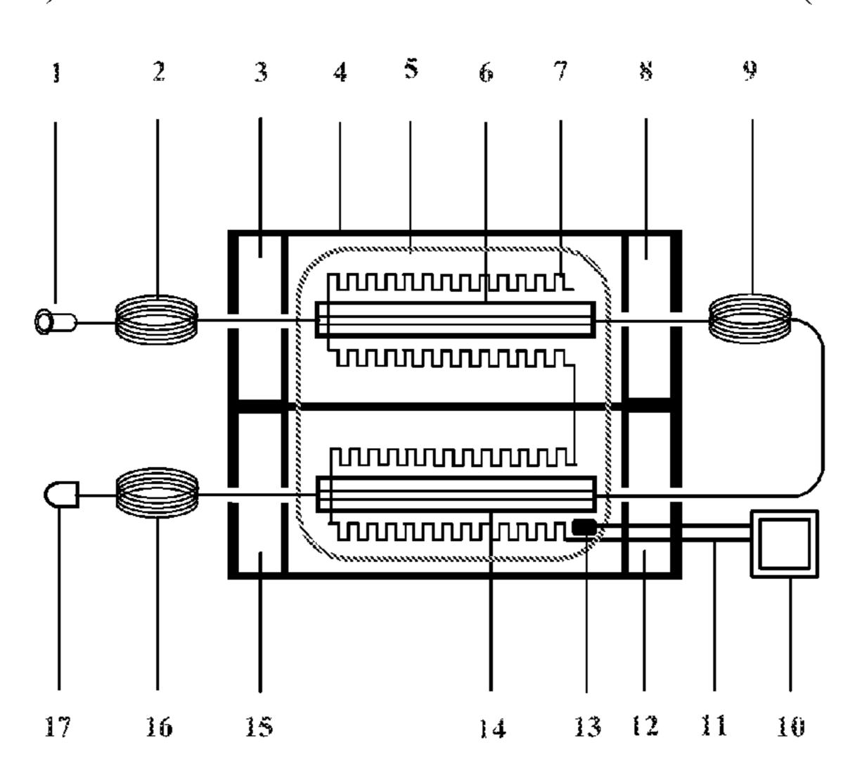
two capillary atomic cells working in the same temperature environment; a polarizing plane changes after interaction between a weak signal light and atoms.
