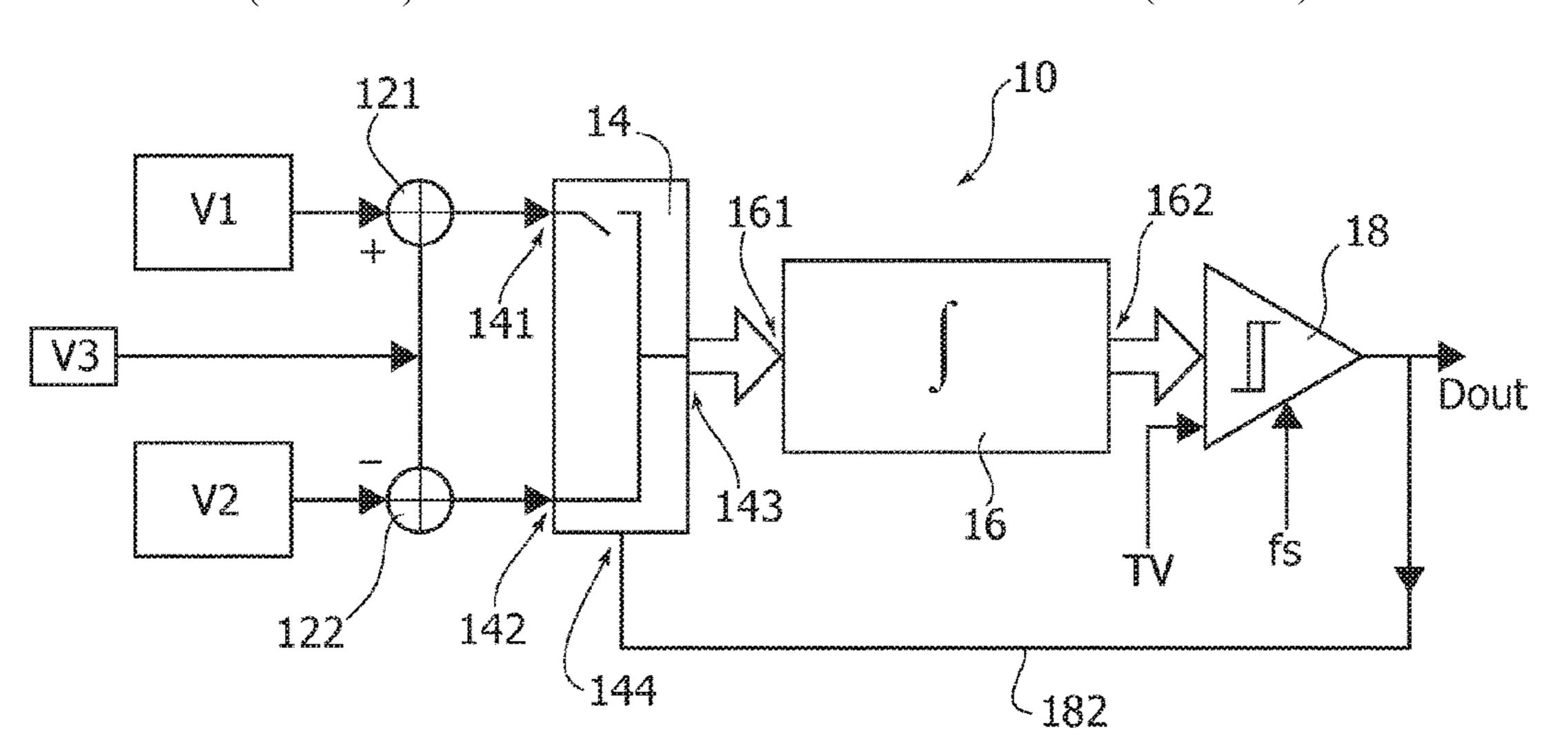
signal and causing the selector to select the subtracted signals in response to the second level of the output signal.
