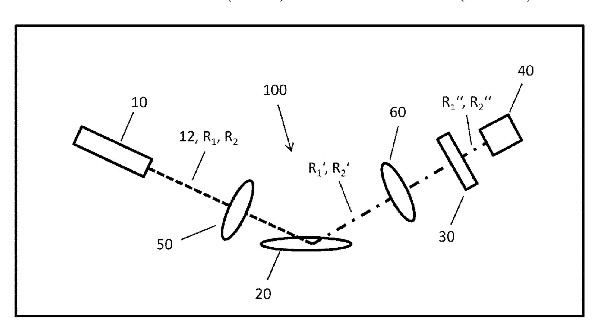
the filter wavelength from the first excitation radiation scattered and filtered by the sample. Additionally, the filter element wavelength-selective filters the second excitation radiation scattered by the sample. A second intensity is determined through the single-channel detector assigned to the filter wavelength from the second excitation radiation scattered and filtered by the sample.
