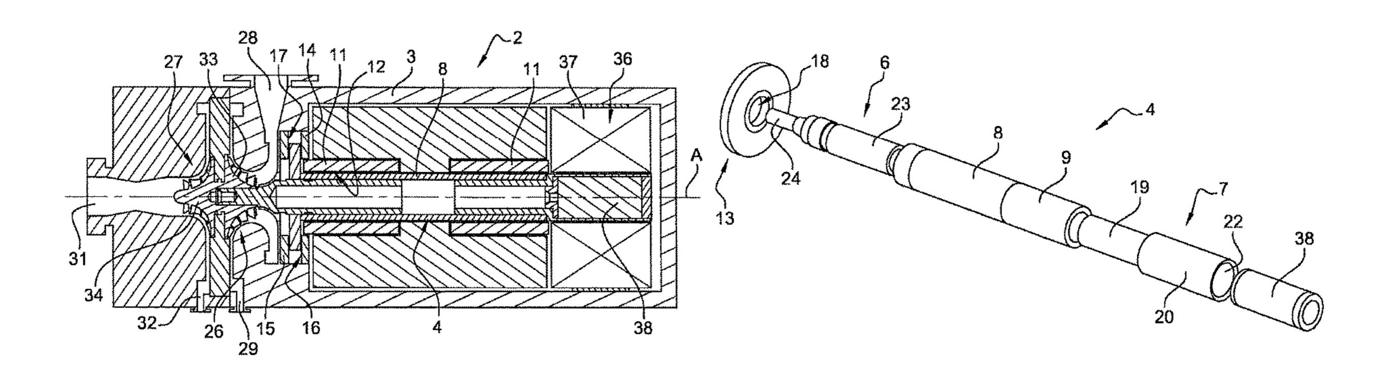
during assembly of the impeller portion (6) and/or the driving portion (7) to the tubular bearing portion (5), are substantially limited to the driving portion (7) and/or the impeller portion (6).
