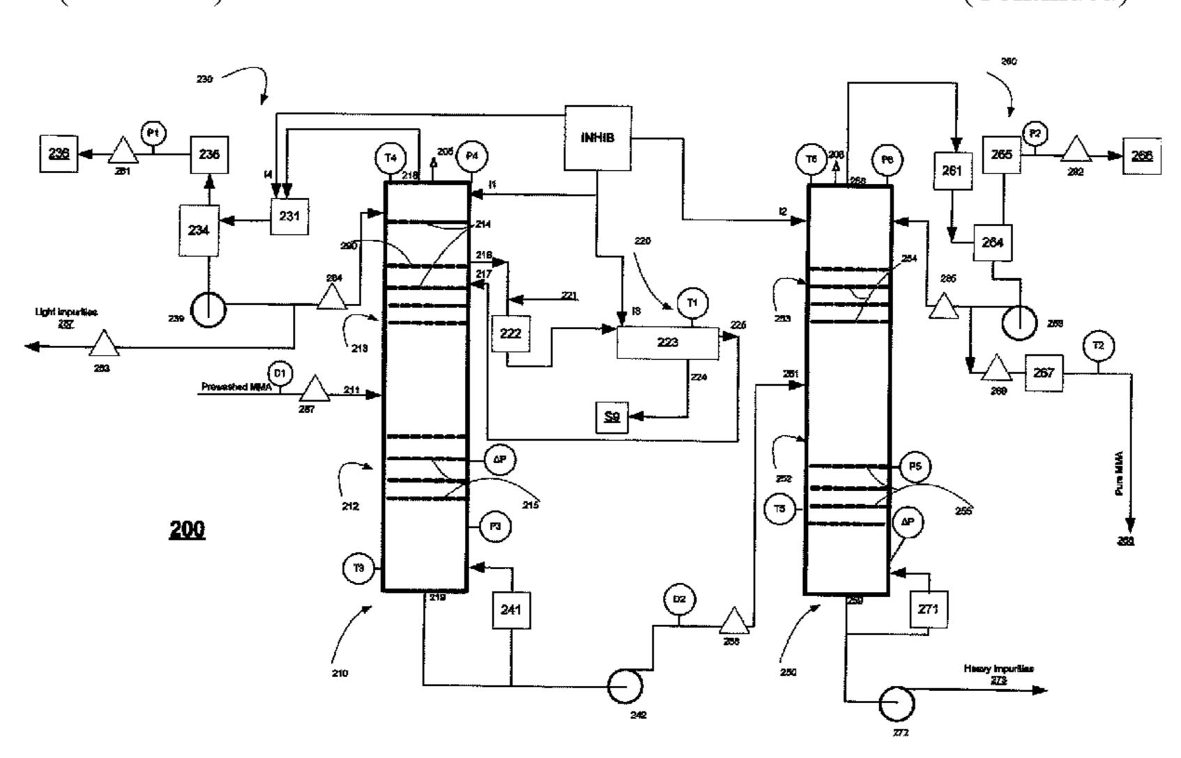
issued from bottom of first distillation column (210). The upper part (213) of first distillation column (210) is connected to a lateral extraction system (220), able to minimize MMA content in light impurities flowing upward said first column (210).
