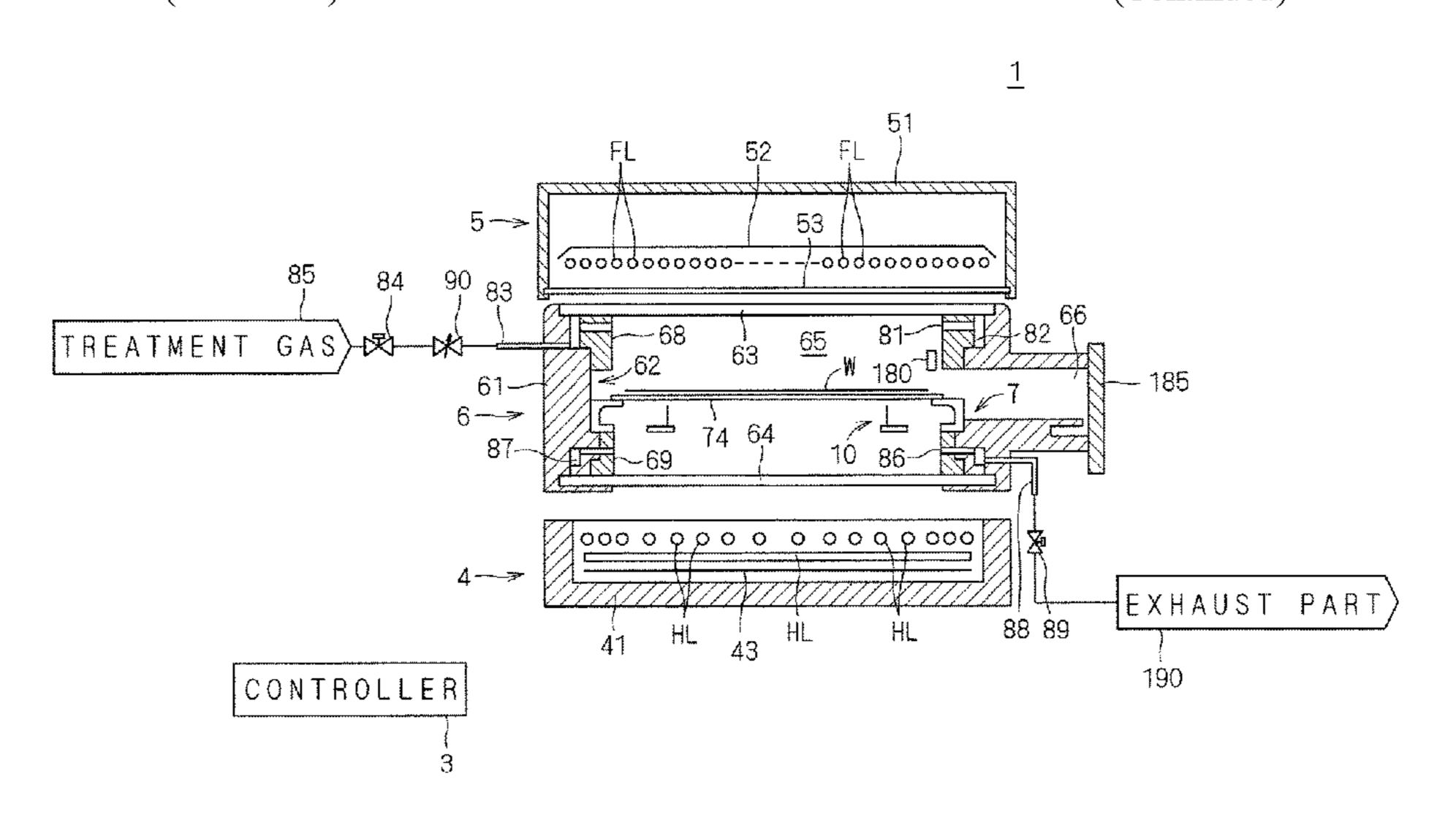
irradiated with a flash light, thereby performing post deposition annealing (PDA) on the high dielectric constant film. Since the pressure is reduced once to be lower than atmospheric pressure and then returned to ordinary pressure, a chamber's oxygen concentration is lowered remarkably during the PDA. This restricts an increase in thickness of the silicon oxide film underlying the high dielectric constant film by oxygen taken in during the PDA.
