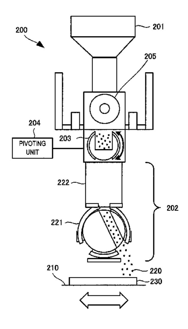
replenishes the powder spreader with a predetermined amount of powder. The pivoting unit of the powder supply apparatus causes the powder replenisher to pivot.
