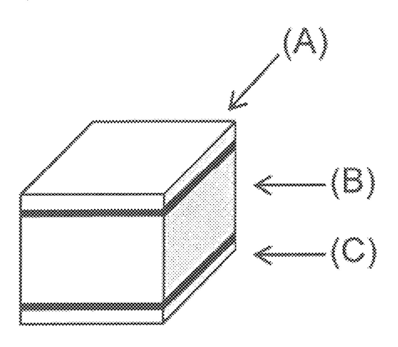
the above-described layer (A) composed of sparingly watersoluble polymer to dissolution of the other outermost layer is 10 seconds to 5 minutes.
