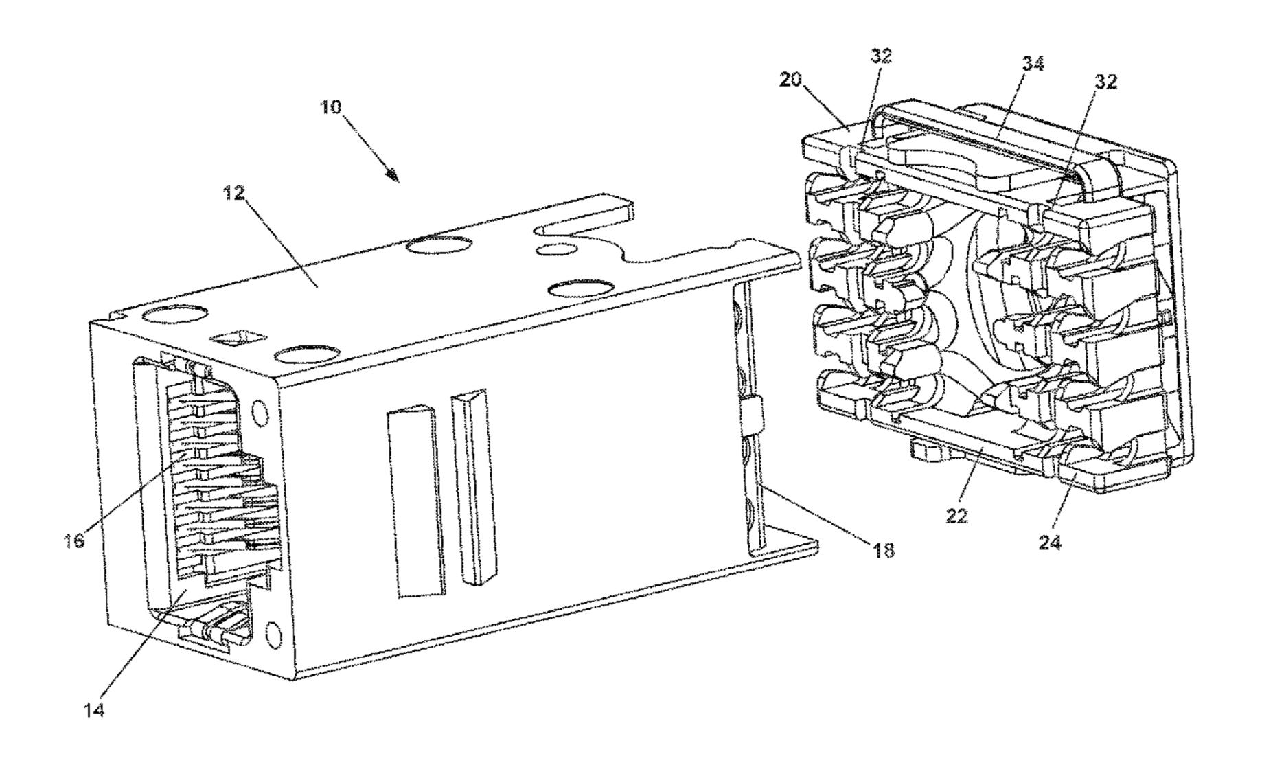
to sever or break the breakaway portions (34) such that the separable lacing fixture (24) is separated from the fully formed connector (10).
