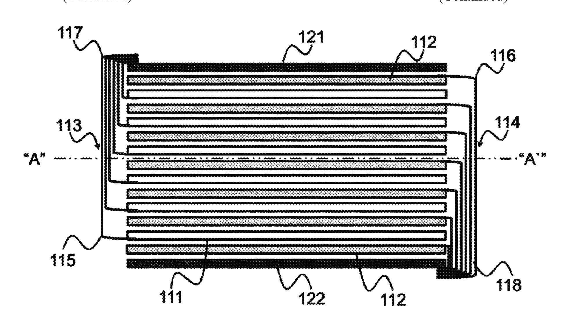
a battery case having a structure of surrounding an external surface of the electrode assembly.
