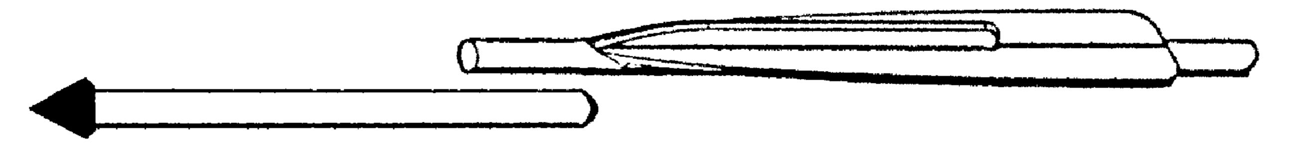
A tubular shaft with point slides over the dowel shaped shaft of the plastic fletch unit creating a pistol crossbow bolt, a crossbow bolt or an archery arrow, depending the length of the tublar shaft.
