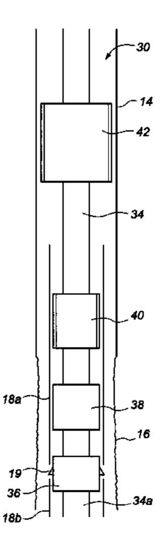
tool and spear tool can be configures to grip the respective casings during cutting of the second casing string. The cut casing section can then be pulled using the downhole pull tool to dislodge the casing section, whereupon via attachment to the spear tool, the cut casing section can be removed from the well. The assembly can be re-set at shallower depths in the event that the cut casing section cannot be dislodged for removal.
