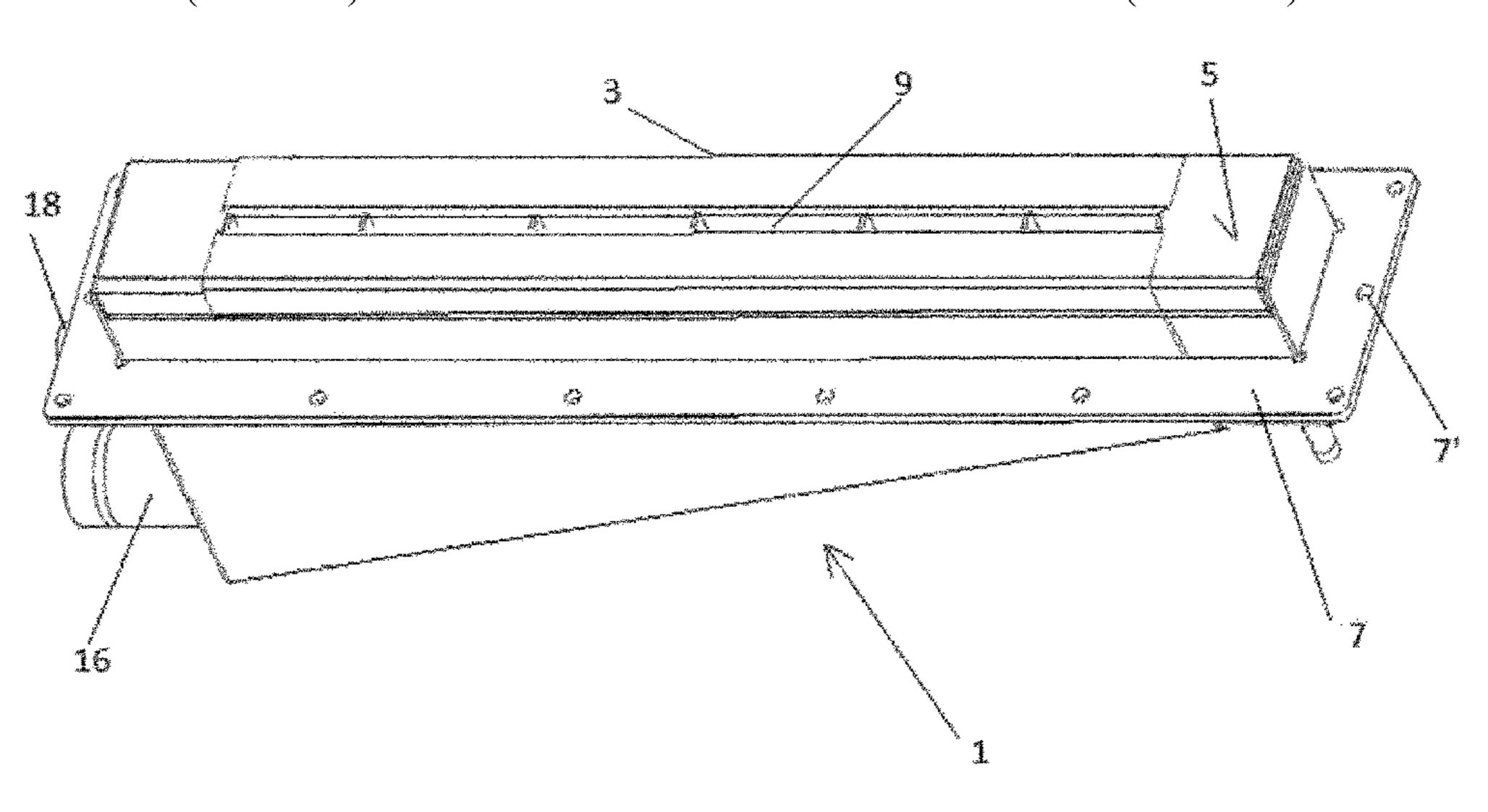
comprising a connection to a supply of oxygen and the other comprising a connection to a supply of fuel gas. The ends of the branches of the longitudinal volumes are connected to the burner nozzles. A flange is arranged around the parallelepipedic burner body at a distance from the melt oriented face of said body.
