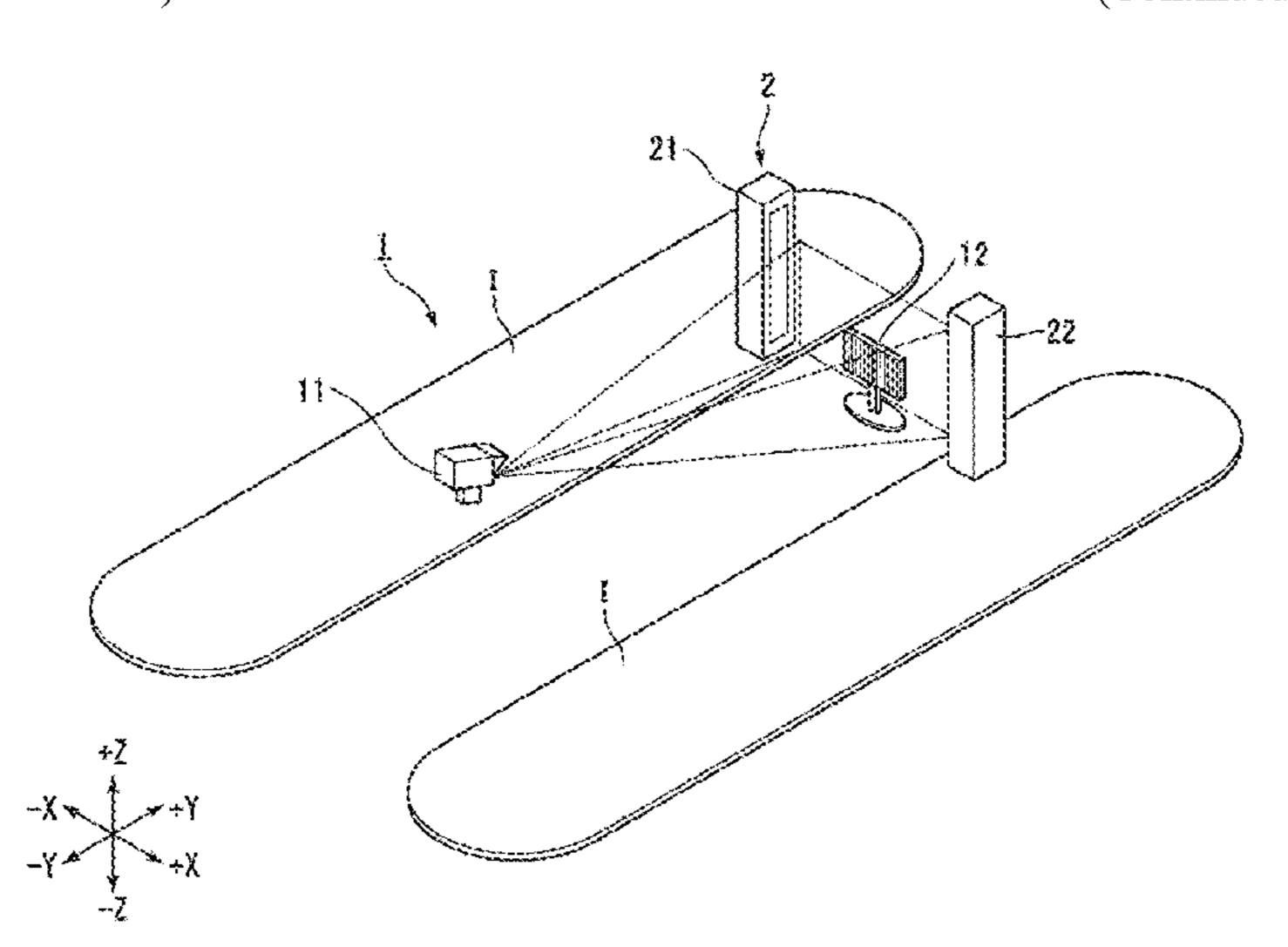
of a plurality of colors provided at the target shooting position comes out. A focusing position determination unit determines a focusing position of the camera based on a change of the evaluation score calculated by the evaluation unit.
