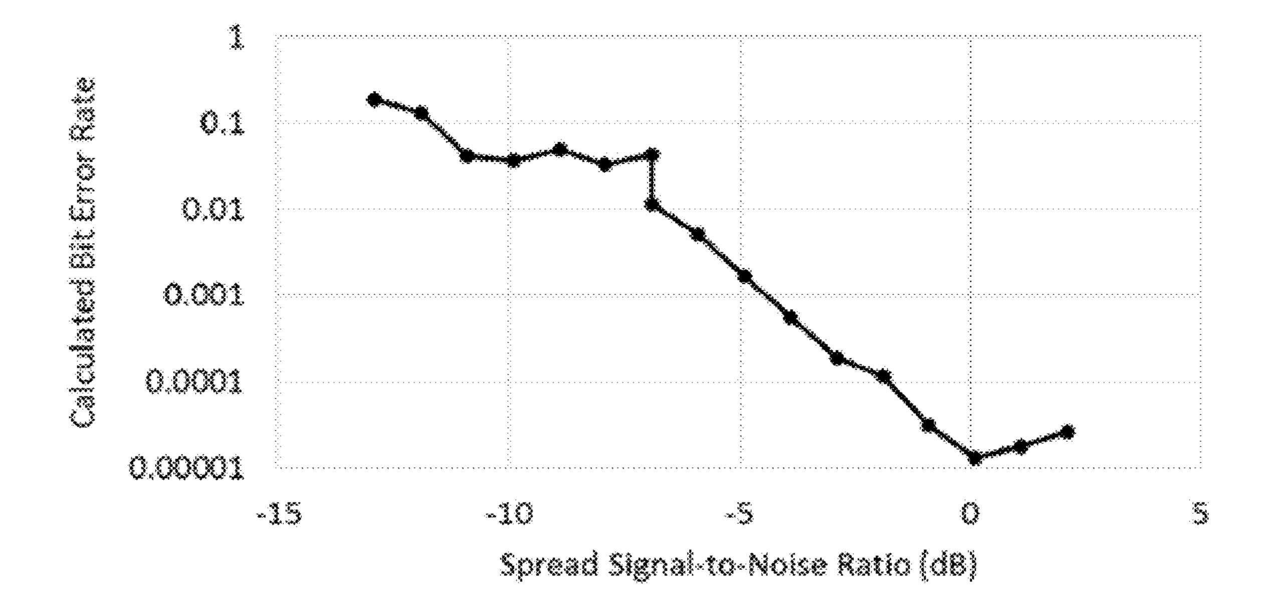
Measured bit error rate versus SNR (E<sub>2</sub>N<sub>0</sub>) for preliminary HOPS hardware testbed
