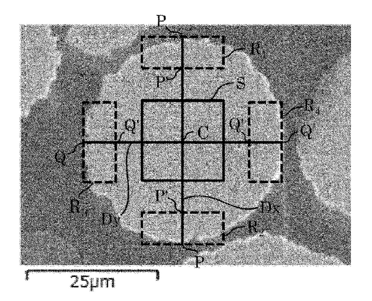
particles containing 15 mass % or more and 25 mass % or less of Mn, 0.5 mass % or more and 5.0 mass % or less of Mg, 0.05 mass % or more and 4.0 mass % of Sr, and 45 mass % or more and 55 mass % or less of Fe, with Si localized in the surface thereof is used.
