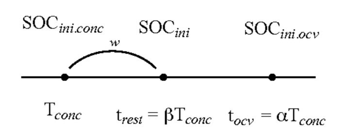
In this example,  $\tau_{conc}$  is the stabilizing time, and  $\tau_{ocv}$  is a sufficient time for the Li ion concentration to reach the equilibrium state, and is  $\alpha * \tau_{conc}$  (ex. 1<\alpha<2). Thus, in this example,  $t_{rest}$  is the determination time point that determines a current initial condition, and is the battery reoperation time point, and  $t_{rest}$  is  $\beta * \tau_{conc}$ .
