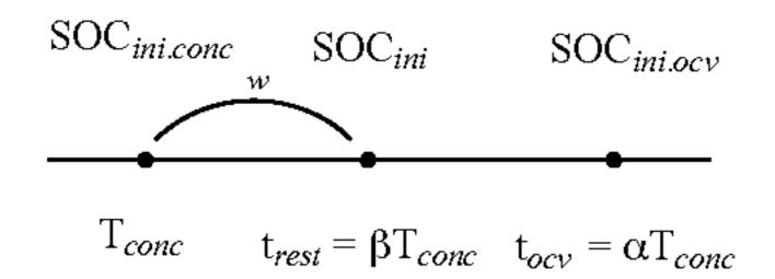
In this diagram,  $\tau_{conc}$  is the stabilizing time, and  $\tau_{ocv}$  is a sufficient time for the Li ion concentration to reach the equilibrium state, and has a value of  $\alpha^*\tau_{conc}$ , for example, 15 such that  $1 < \alpha < 2$ . In such an example, t is the determination time point that determines a current initial condition, and may be the battery reoperation time point, and  $t_{rest}$  is  $\beta * \tau_{conc}$ .
