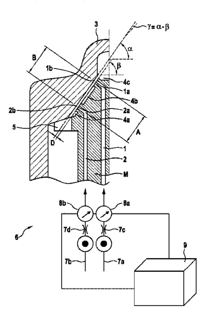
admittedly high precision of pneumatic length measurements can be converted in a particularly advantageous manner to high precision of the angle measurement in this manner. The tilt angle can be measured at least with an accuracy of less than one tenth of a degree. At the same time, the measurement is fast enough for 100% control in mass production. The plug gauge is the central element in the measuring system and in the method, to which the invention likewise relates.
