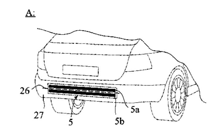
direction with the aid of a motor upon detection of a primary operator occurrence via the operator occurrence sensor. Further the cargo compartment device comprises at least one motor-displaceable cargo compartment component and the control arrangement displaces at least one such cargo compartment component with the aid of a motor upon detection, via the operator occurrence sensor, of a secondary operator occurrence following the primary operator occurrence.
