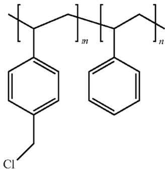
The membranes were prepared by casting the PSMMIM solution prepared above directly onto a flat glass surface. The thickness of the solution on the glass was controlled by a film applicator (MTI Corporation, Richmond, Calif.) with an adjustable doctor blade. The membranes were then dried in a vacuum oven at 80° C. for 300 minutes, and then 120° C. for 200 minutes. Chloride ion in the membranes was removed by soaking the membranes in 1 M KOH solution for 24 hours.
