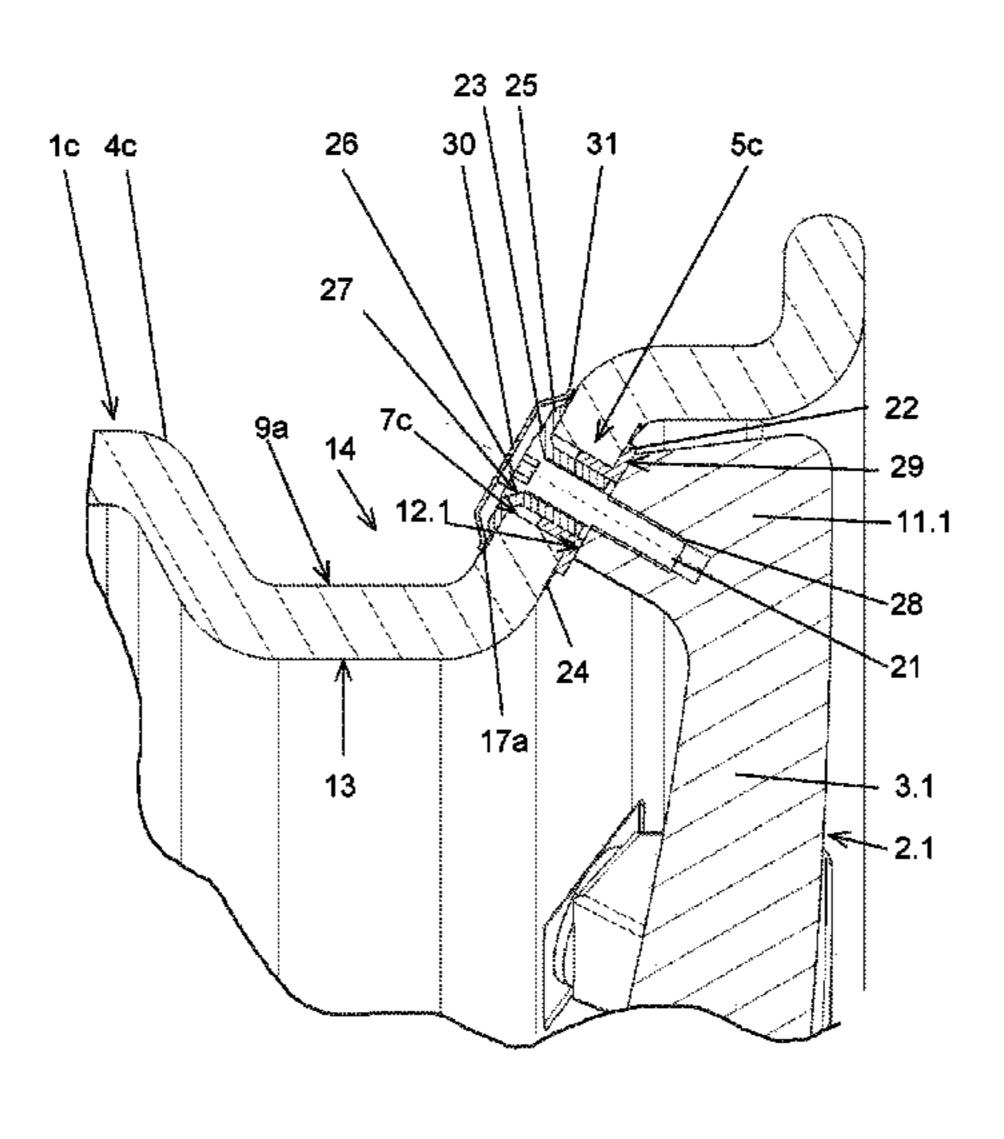
rim comprises a connecting arrangement with a connecting element and a flexible sealing layer made from plastic and completely covers, by coating, a part of the connecting arrangement which extends over the rim outer side of the rim base. An edge region of the flexible seal layer is connected in an air-tight manner to the rim base.
