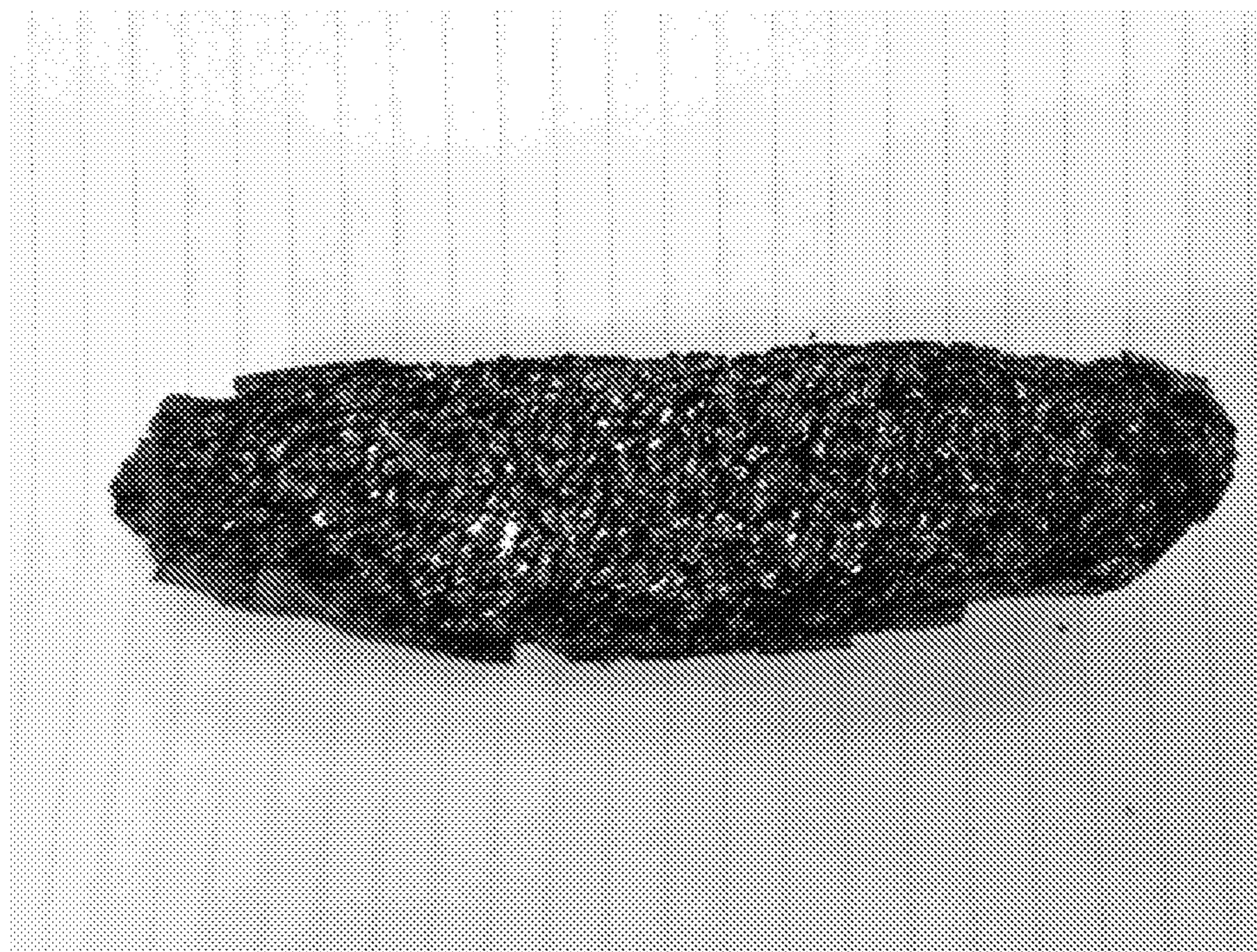
Figure 14 100% lignin monolith after pyrolysis
