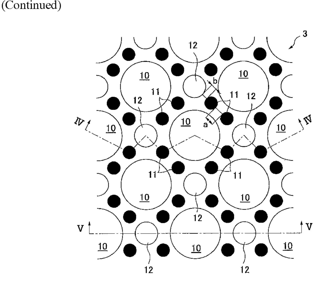
four sides of which are surrounded by the protruding parts (10), and the embossed parts (11) are continuously or non-continuously arranged, between the adjacent opening parts (12), along directions that connect the adjacent opening parts (12).
