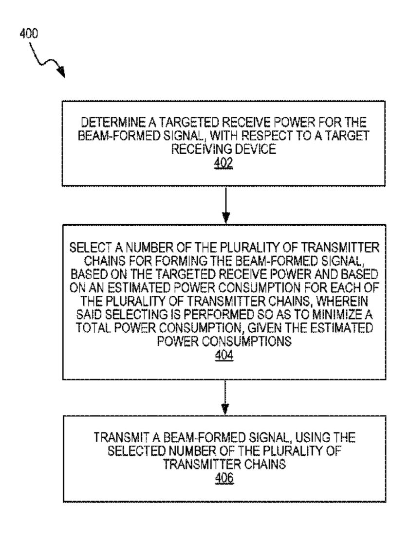
power consumptions. The wireless device transmits a beamformed signal, using the selected number of the plurality of transmitter chains.
