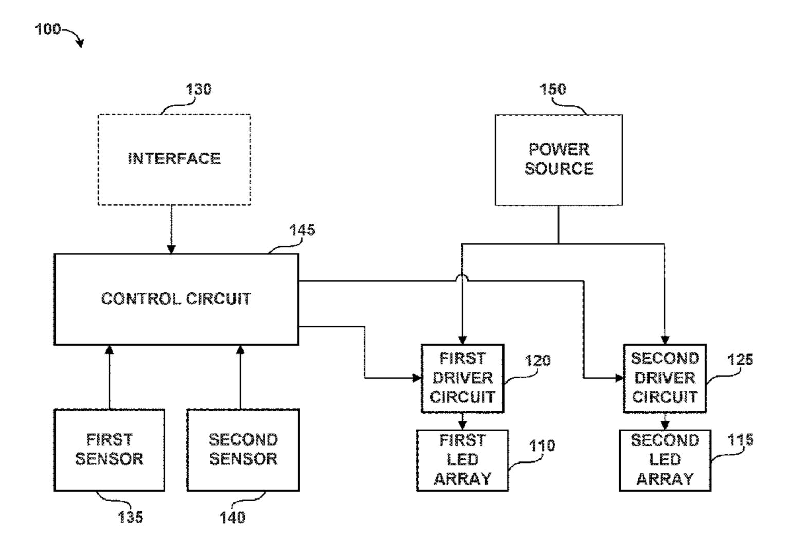
sensors and to control the first LED array and the second LED array based on the signals.
