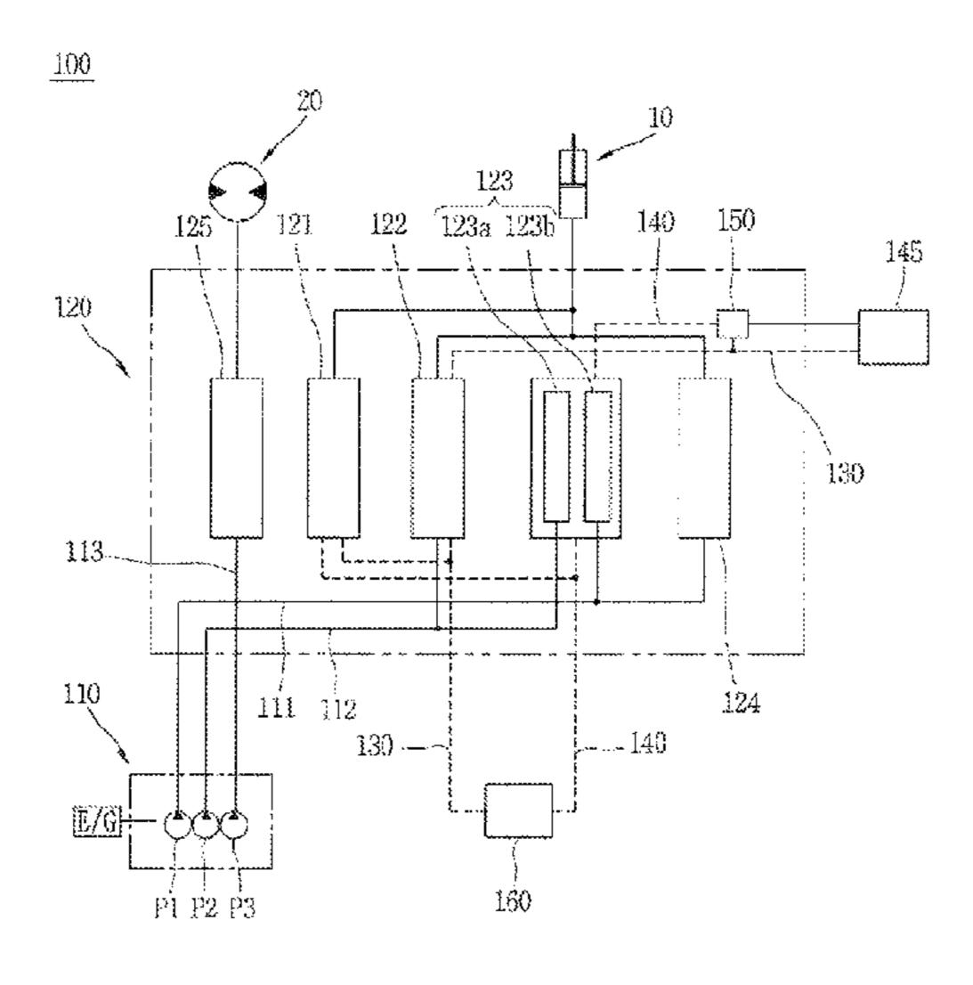
a tank, that is connected to the first pilot signal line, and that is switched when the operation apparatus spool is switched so as to cut off the flow of a pilot pressurised fluid that is returning to the tank.
