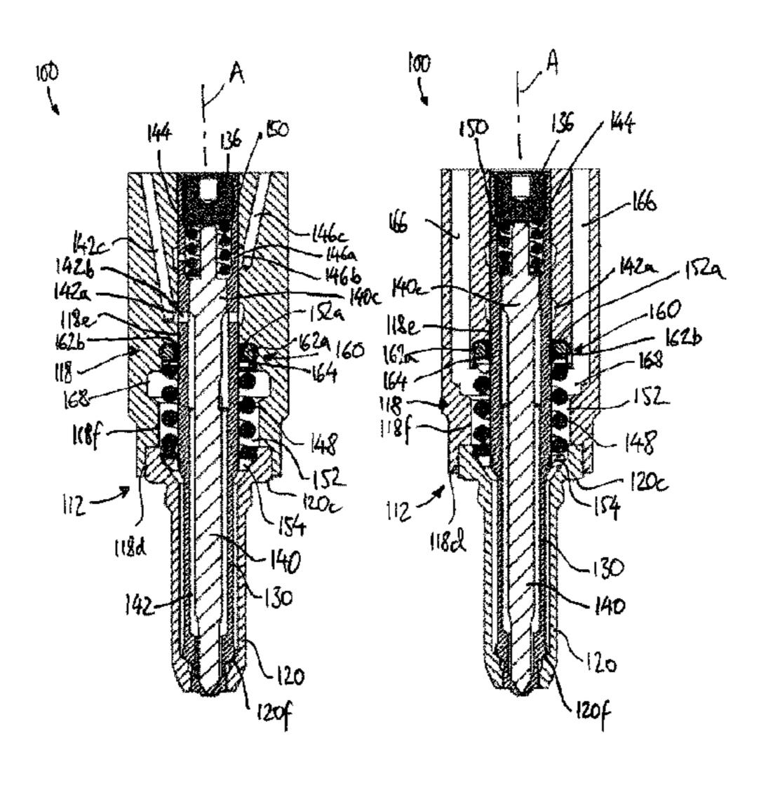
valve needle and a fuel. A collar for seating the biasing spring can be dimensioned to allow free flow of the fuel from the cavity into an annular accumulator volume defined between the outer valve needle and the bore of the tip part.
