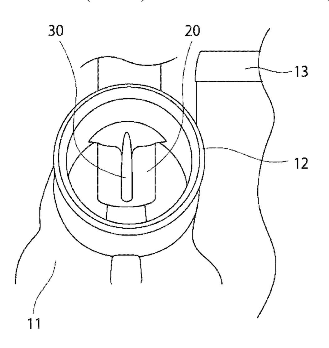
boss opposite the side facing the fluid inlet is provided with a rib.
