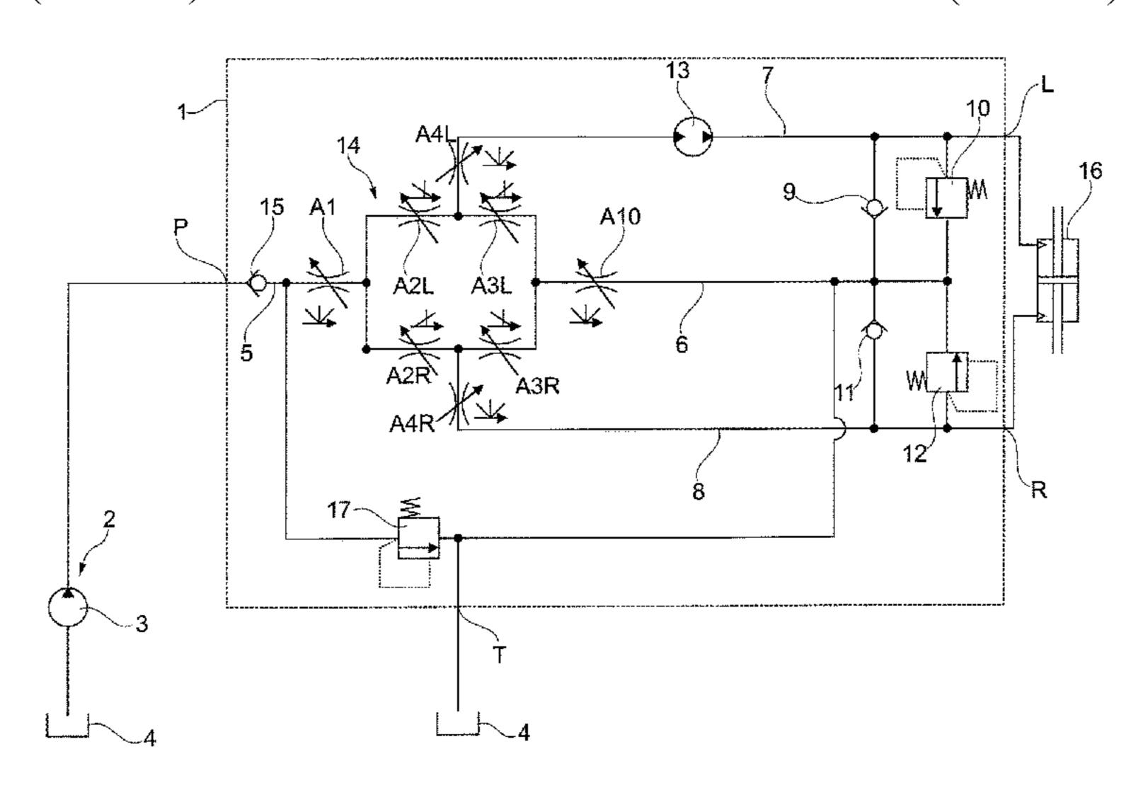
arrangement and the working port arrangement (T), which further orifice arrangement is closed in neutral position.
