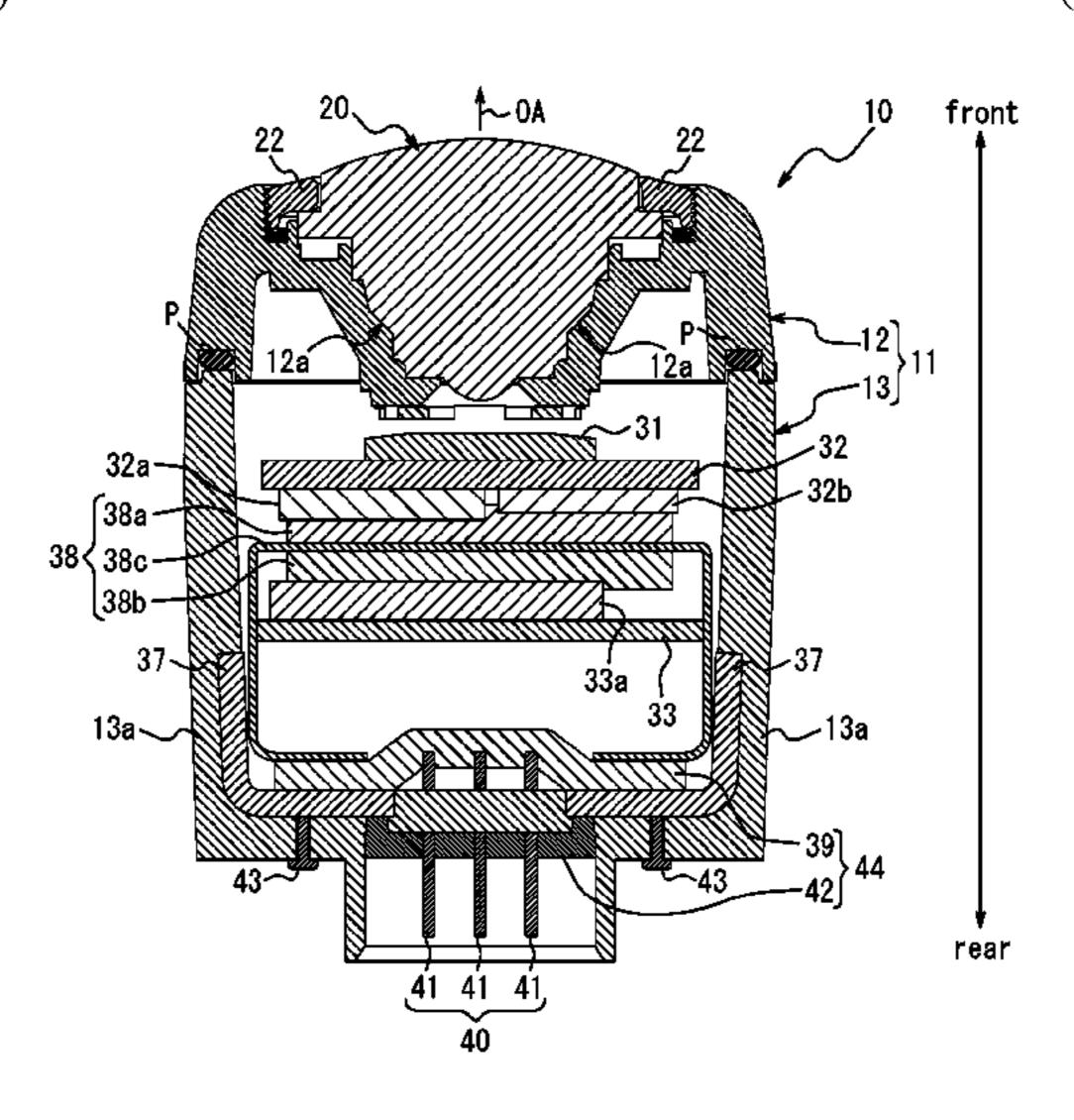
transfer unit that transfers heat generated from at least one of the image sensor and the electronic component to the plurality of terminals.
