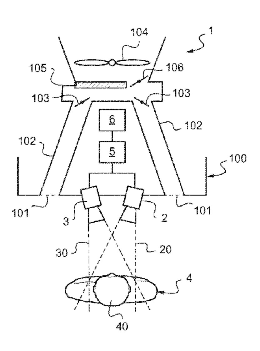
on the images of the first camera (2) and of calculating, from said measurements, at least one thermal comfort coefficient of at least one occupant (4) of the motor vehicle, the thermal comfort coefficient being used for regulating the air temperature, the air flow rate and the air distribution within the heating, ventilation and/or air conditioning system, the control system (1) further comprising a second camera (3) sensitive to wavelengths in the visible and/or near-infrared spectra.
