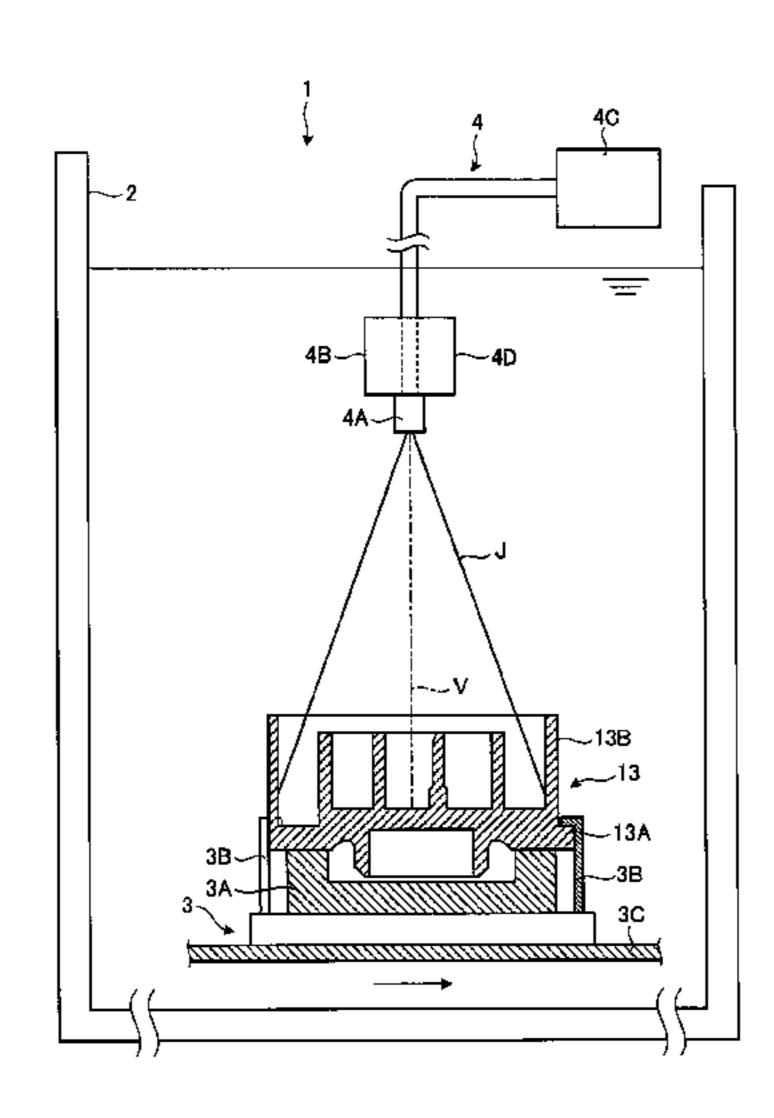
jetting cavitation bubbles generated underwater by a water jet at a first side of an end plate (13A) of the scroll (13), with a center (P1, P2, P3) of the cavitation bubbles being offset from a center (O) of the spiral shape of a wall portion (13B) on the end plate (13A) and the step portion (13Aa) and the stepped portion (13Ba) positioned at an outer peripheral portion of the cavitation bubbles (C).
