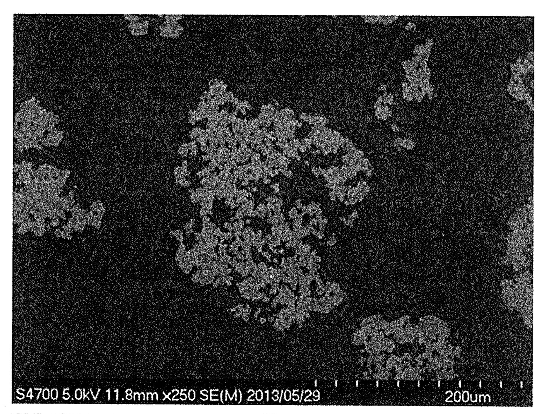
AFTER PERFORMING HYDROGEN REDUCTION REACTION THREE TIMES
