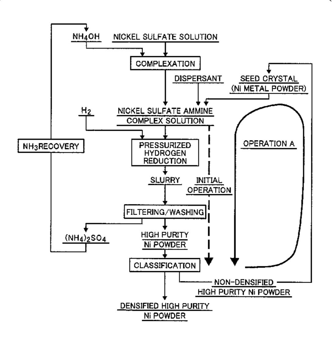
temperature of the solution, and performing a reduction reaction with hydrogen by blowing hydrogen gas into the pressure vessel, thereby obtaining the nickel contained in the nickel ammine complex solution as nickel powder; and thereafter, performing a specified operation A repeatedly at least once to obtain the nickel powder having the median diameter of 100 to 160  $\mu$ m and a bulk density of 1 to 4.5 g/cm<sup>3</sup>.
