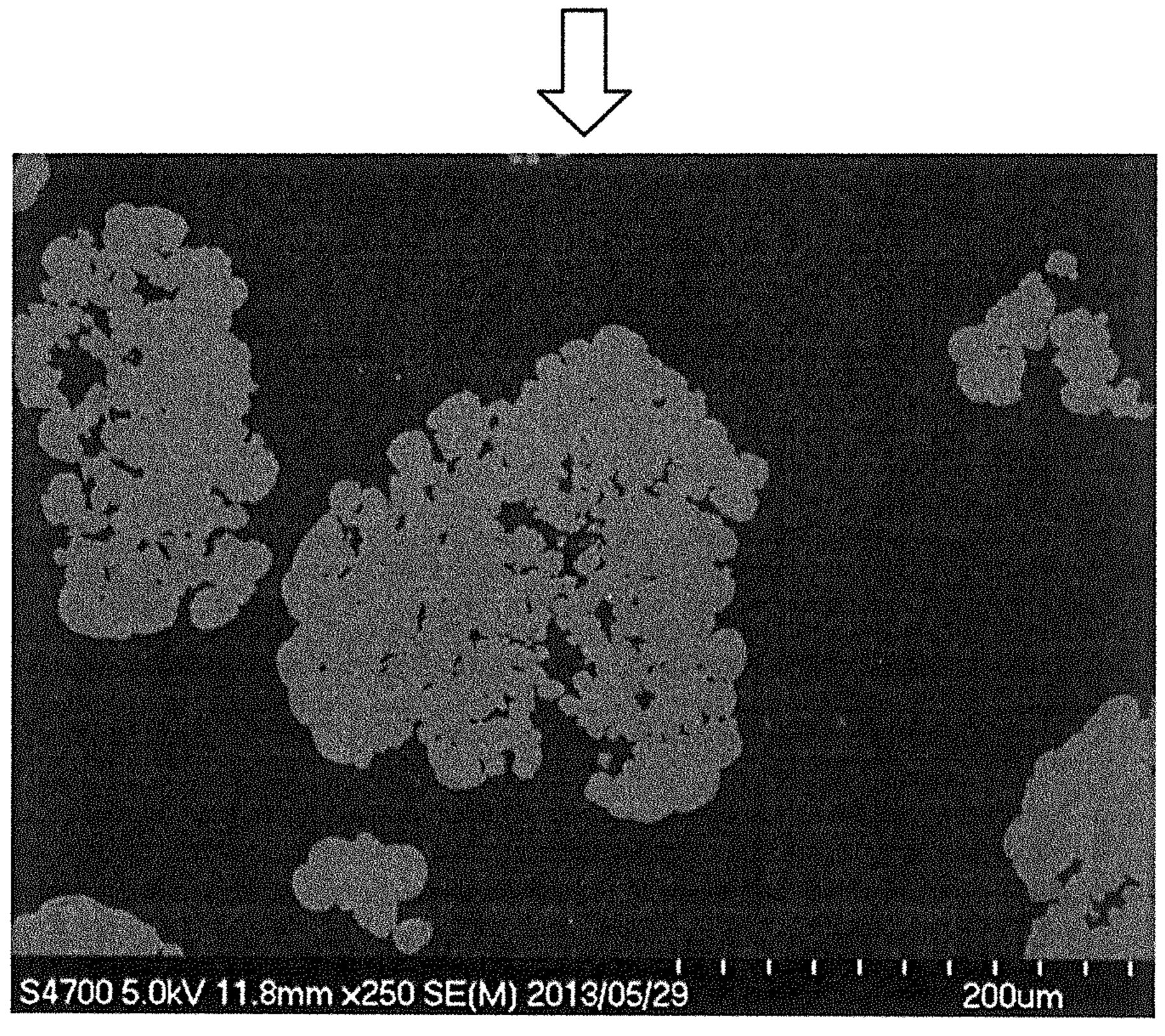
AFTER PERFORMING HYDROGEN REDUCTION REACTION FIVE TIMES
