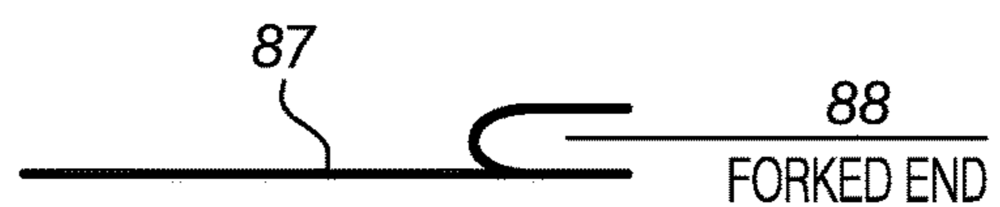
SIDE VIEW OF TWO PRONGED PUSHER 87
