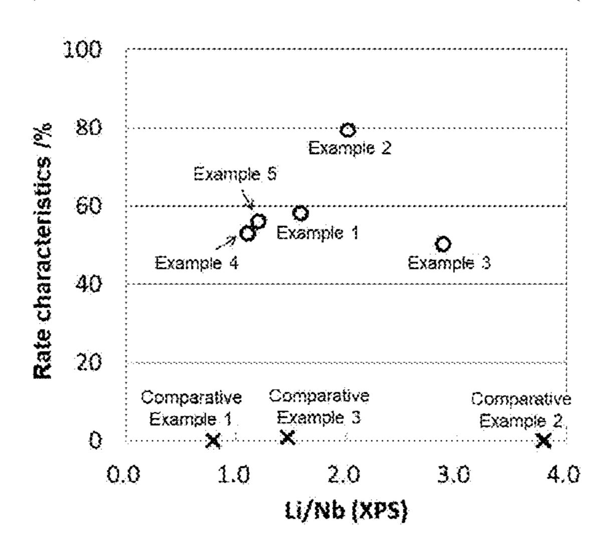
ondary battery, wherein the surface of present core particles composed of a spinel-type composite oxide containing Li, Mn, O, and two or more other elements is coated with an amorphous compound containing Li, A (A represents one or more elements selected from the group consisting of Ti, Zr, Ta, Nb, and Al), and O; and the molar ratio (Li/A) of Li relative to the A element in the surface, as obtained by XPS, is 1.0 to 3.5.
