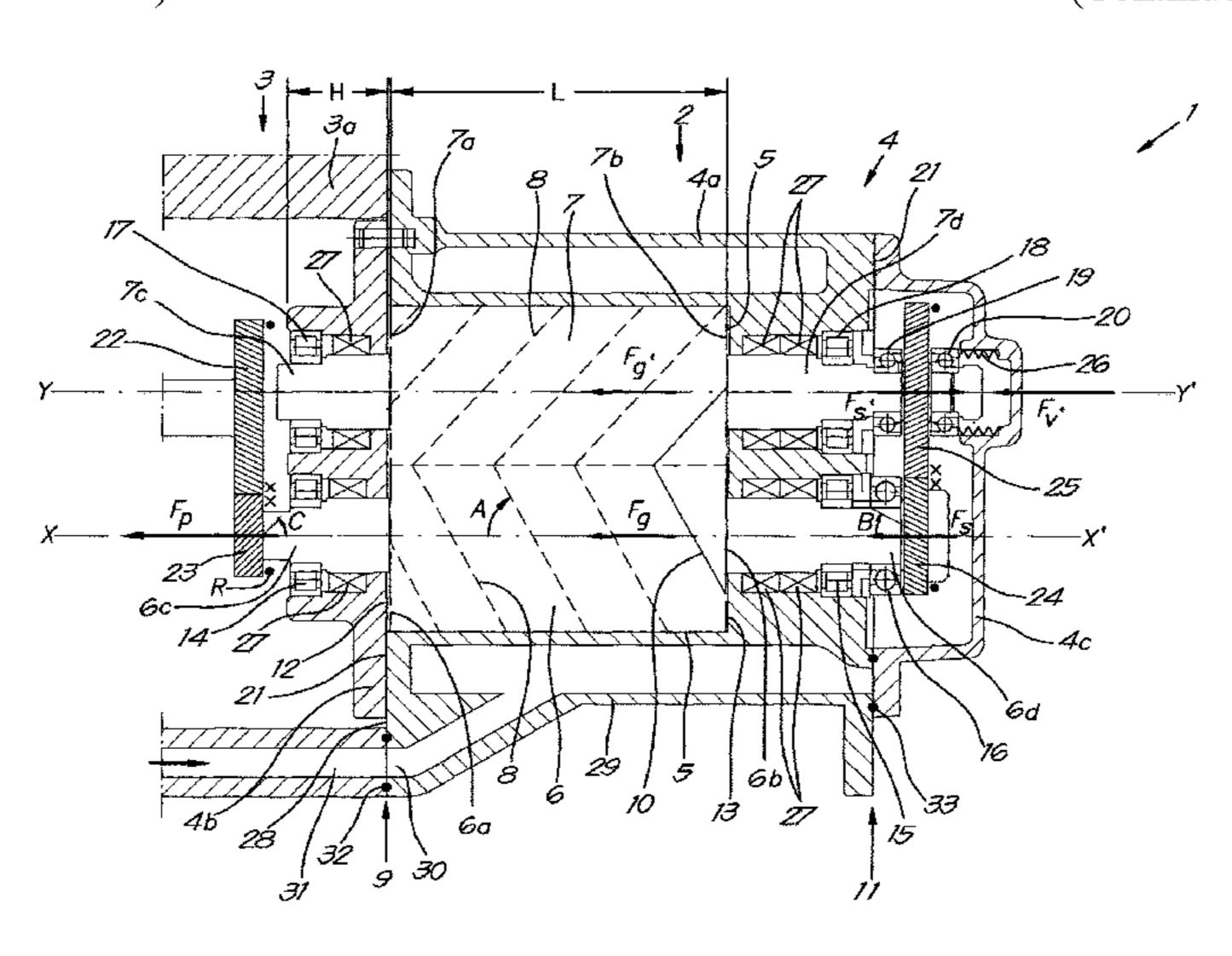
wheels of the male rotor are chosen such that, upon being driven with acceleration of the rotors without gas forces, the resulting mechanical drive force that is exerted by this drive and by this synchronisation gearwheel on the male rotor has an axial component that is directed from the outlet side to the inlet side and that the movement of the male rotor in the axial direction from the outlet side to the inlet side is fixed by means of a single axial single-acting or double-acting bearing.
