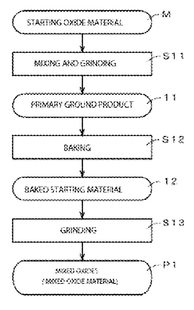
components but containing neither Cr nor Co as a main component, wherein the contents of La, Mn and Cu in the mixed oxides satisfy the following ratios, as oxide equivalent amount with respect to 100% by weight of the oxide equivalent amount: the La content as La<sub>2</sub>O<sub>3</sub> being 35-70 wt %; the Mn content as MnO<sub>2</sub> being 25-60 wt %; and the Cu content as CuO being 0.5-10 wt %.
