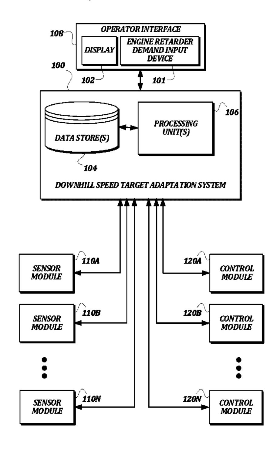
demand in the engine retarder of the vehicle. In response, the system decreases the engine retarder demand setting and, if cruise control is active, increases the DSC cruise control offset.
