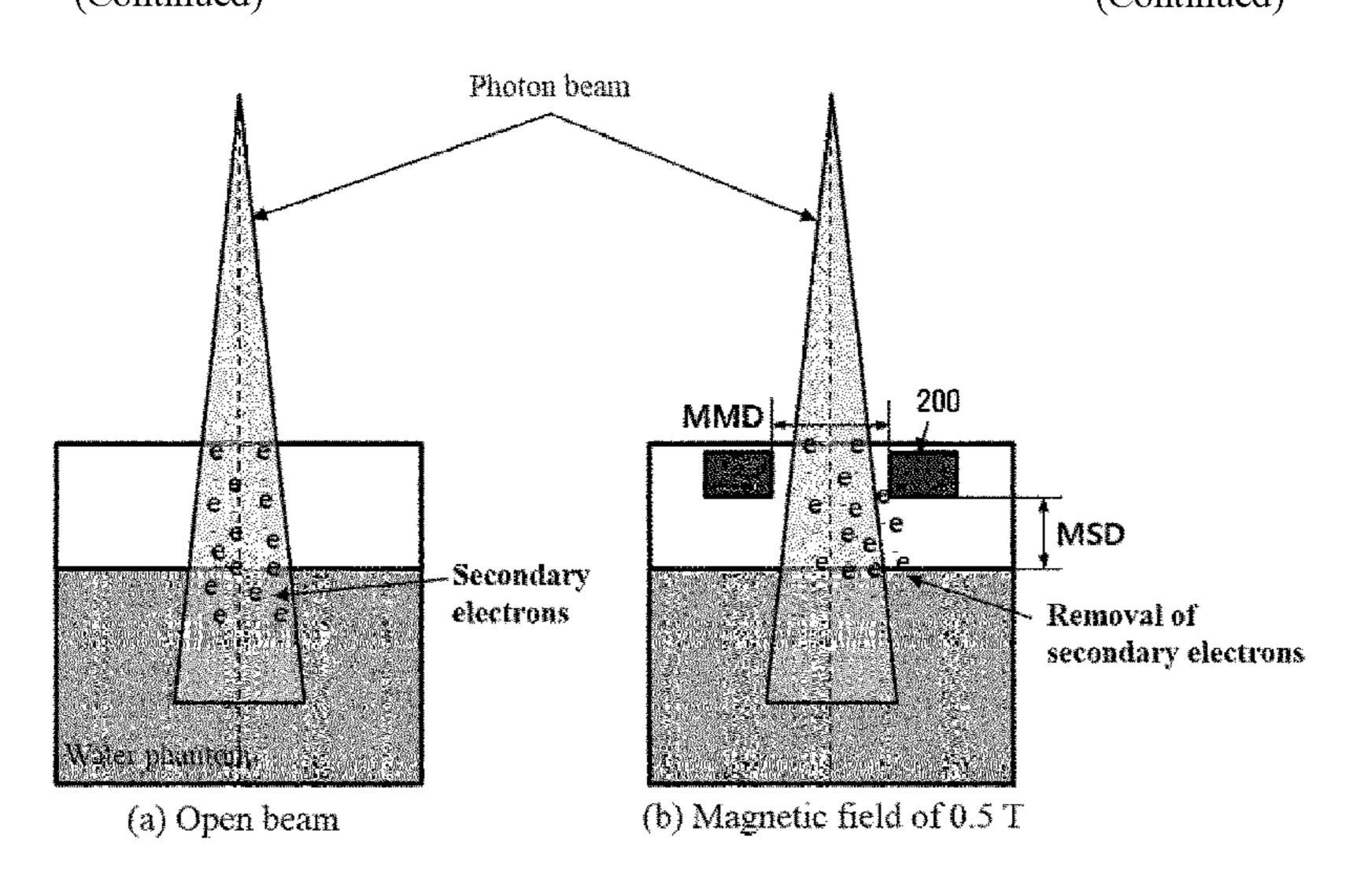
magnetic field intensity adjuster that adjusts an intensity of the magnetic field generated by the magnetic field generator. The magnetic field generator disperses secondary electrons that have particular energy levels equal to or lower than a preset value.
