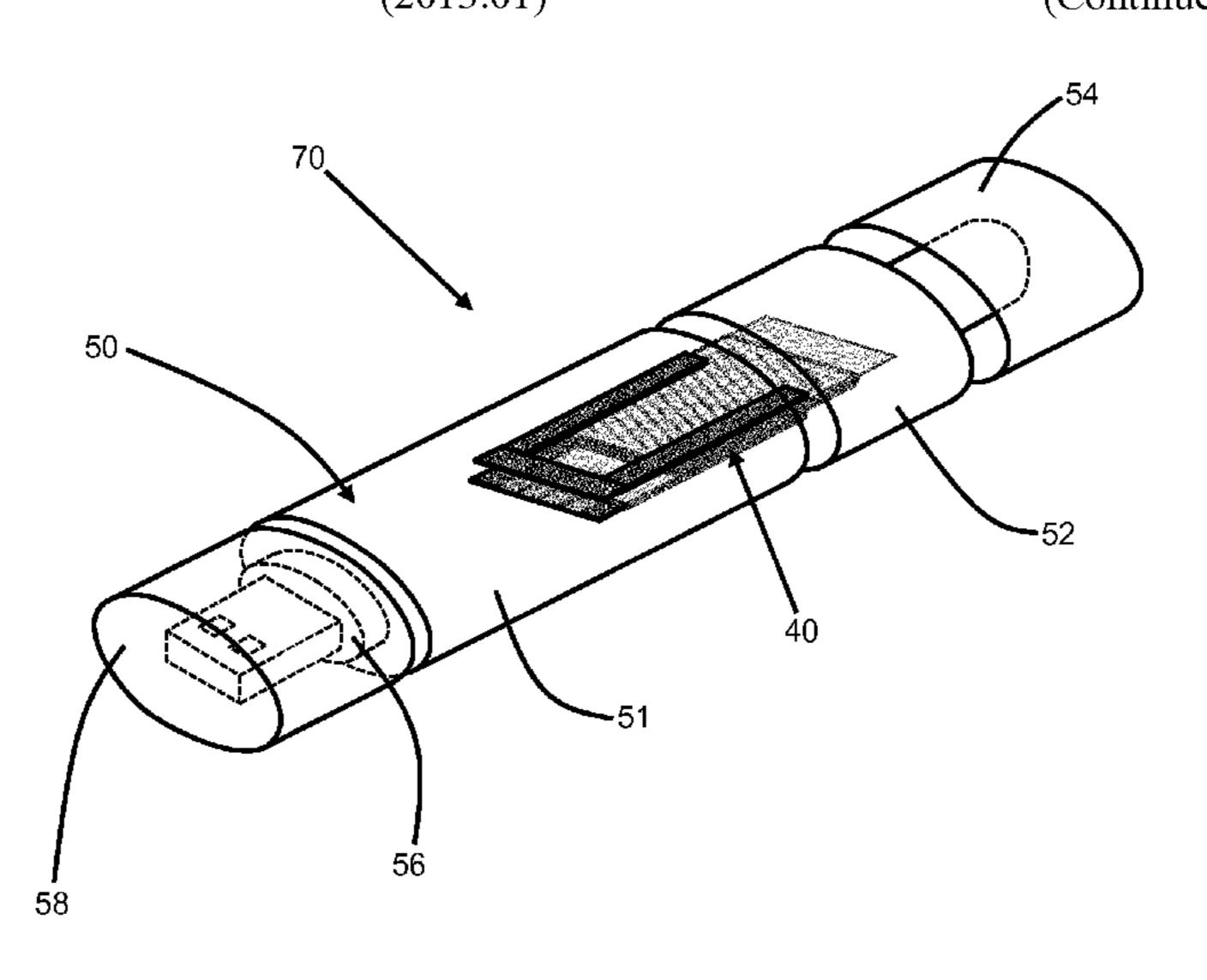
configured to heat the substrate, the cartridge and the heater are substantially flat, and the cavity, the cartridge, and the heater are arranged so that the cartridge and the heater are substantially parallel and adjacent to each other.
