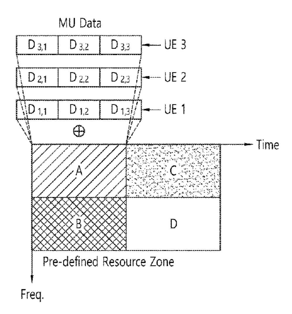
predefined contention zone patterns on the basis of the selected terminal class. The uplink data is transmitted to the base station through a plurality of contention zones included in the selected contention zone pattern.
