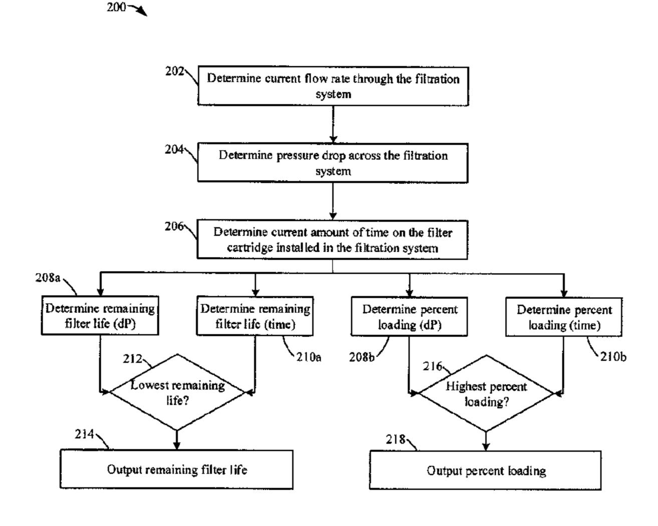
time-based manner (e.g., based on the installation date of the filter cartridge and filter cartridge life specifications) and a pressure differential based manner (e.g., based on a determination of pressure drop across the filter cartridge).
