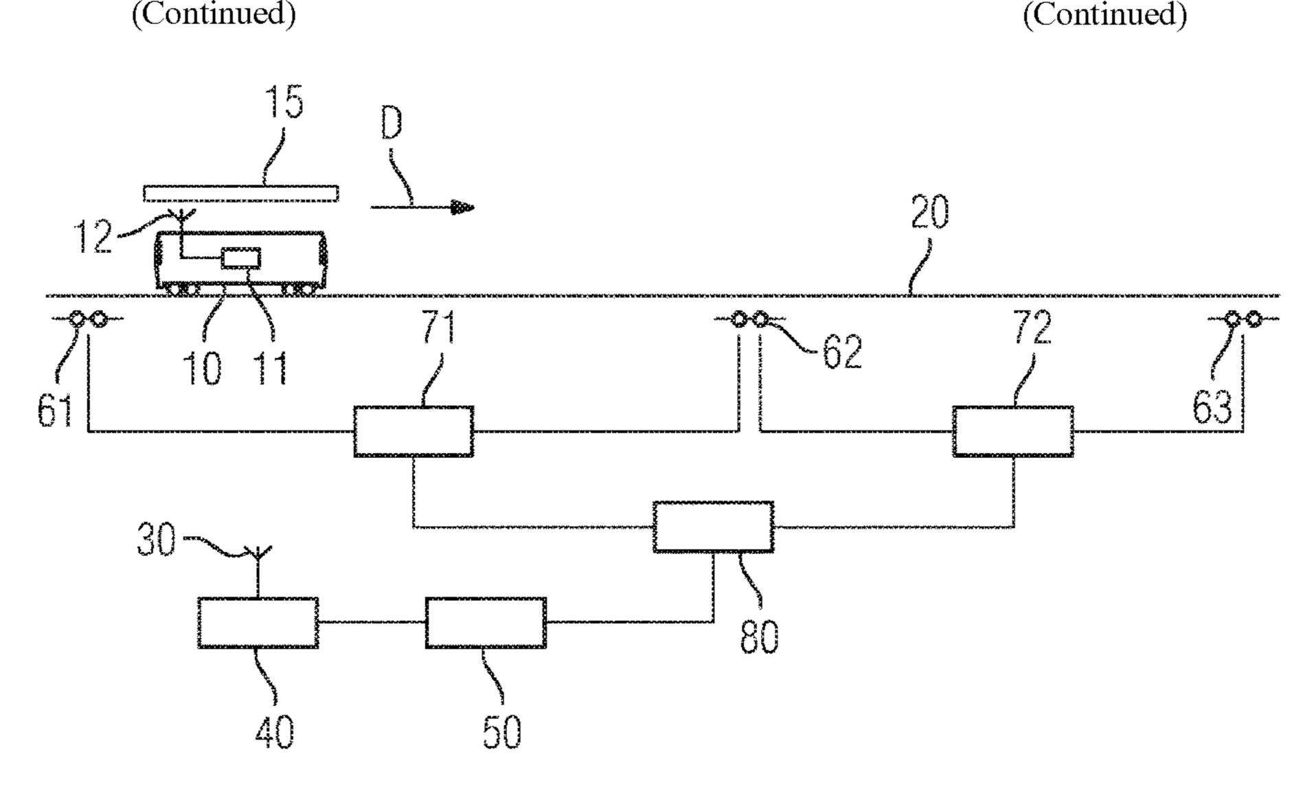
section according to the system. If the vehicle is located completely in the relevant section and the number of axles of the vehicle matches the number of axles located in the section according to the system, a movement authority is ascertained for the vehicle. The part of the relevant section in front of the vehicle in the driving direction is assumed to be free of other vehicles when ascertaining the movement authority.
