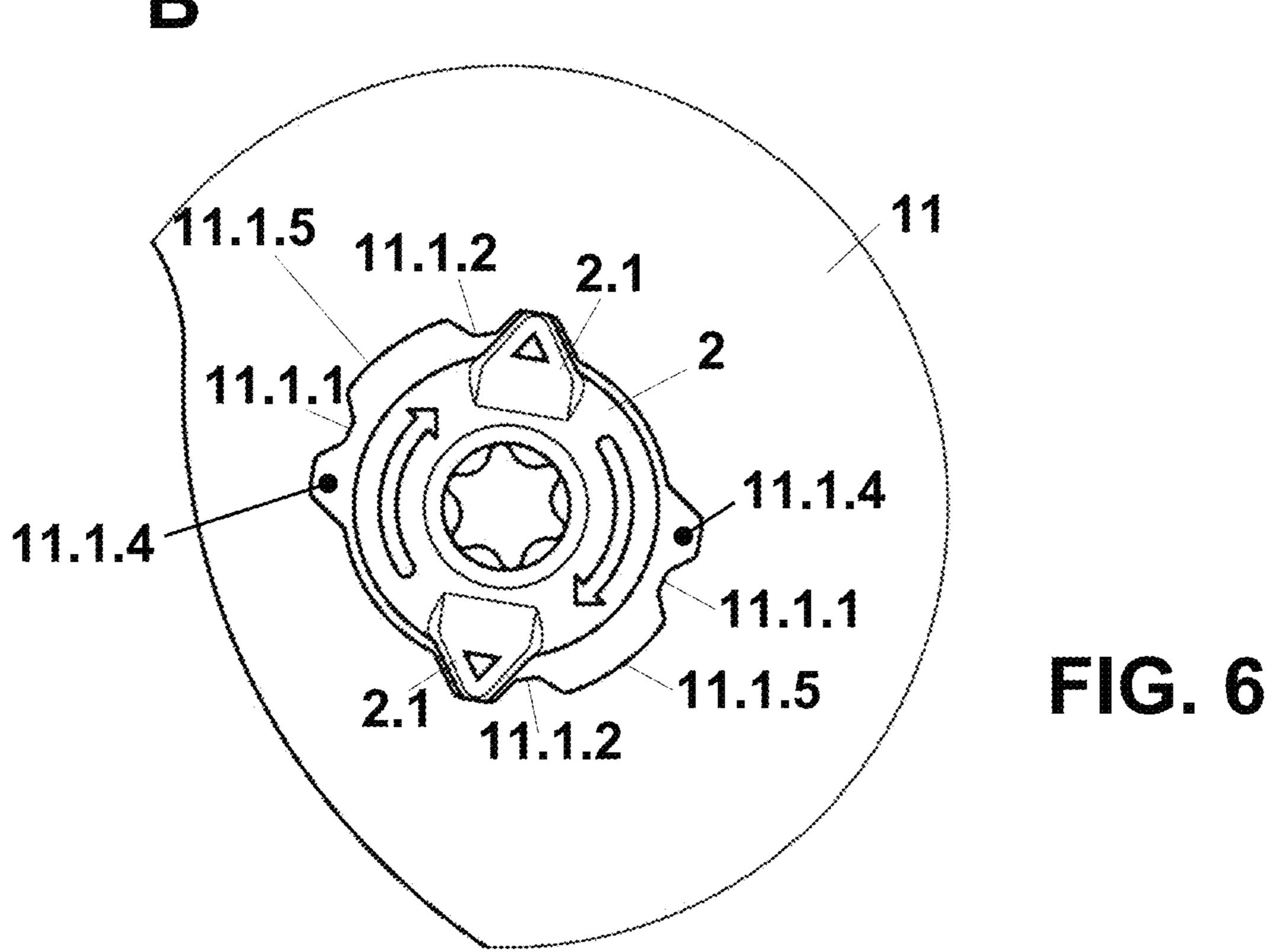
QUARTER TURN CLIP FOR CONNECTING A VEHICLE METAL SHEET PLATE AND AN EXPANDED POLYPROPYLENE VEHICLE PANEL AND QUARTER TURN CLIP AND EXPANDED POLYPROPYLENE VEHICLE PANEL ASSEMBLY
