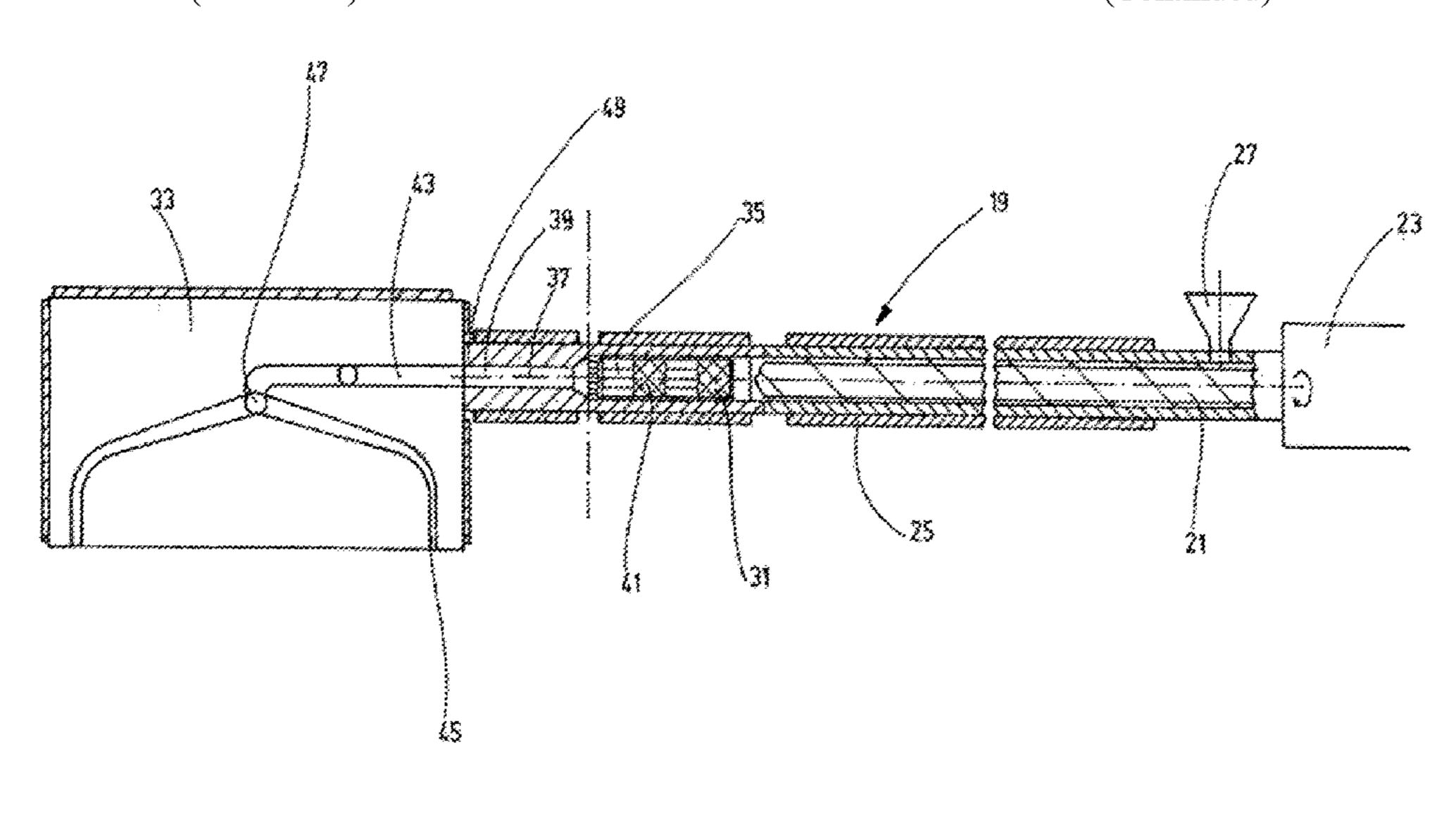
channel guide (41) for the melted plastics material, so that microbiological contaminants are guided predominantly into the interior of the wall of the polymeric tube that interior is enclosed by regions of the plastic material that are less contaminated.
